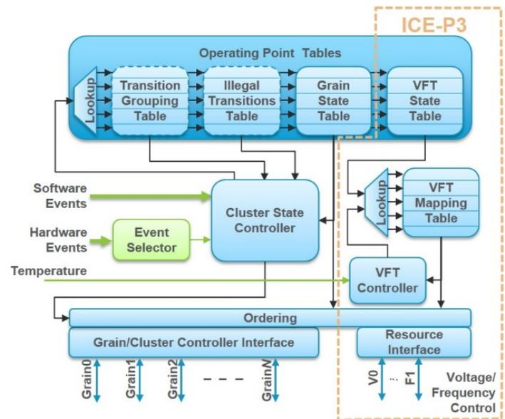
ICE-G3 Cluster Controller / ICE-P3 Operating Point Controller Block Diagram
