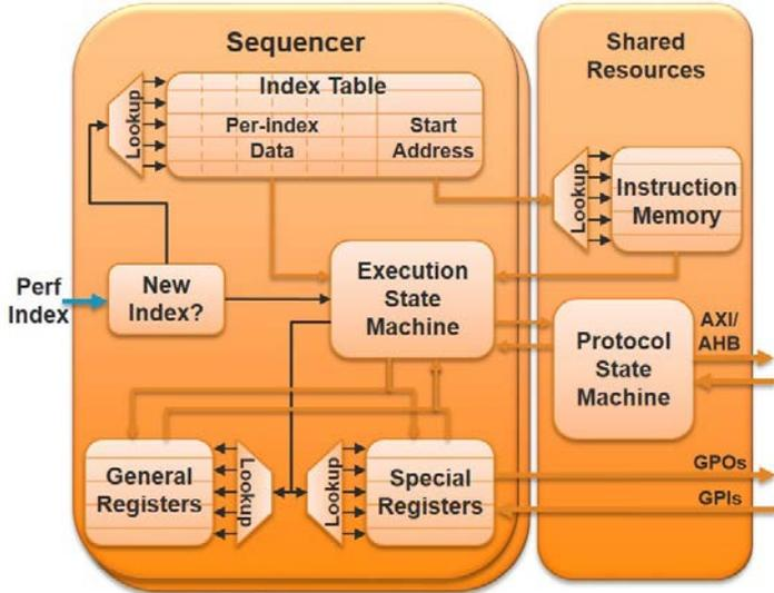
Voltage/Frequency Control Sequencer Block Diagram
