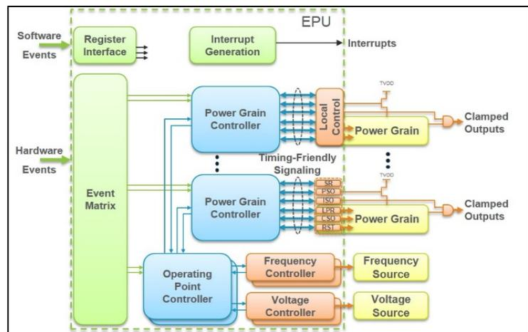
ICE-Grain EPUs are hardware subsystems that manage and control circuit idle moments to minimize energy consumption and maximize power savings. These EPUs are user-configurable and scalable to meet design specifications while providing automated RTL and UPF code generation, verification, and design flow integration with industry-standard EDA environments. ICE-Grain EPUs co-exist and interoperate with conventional approaches to on-chip power management.
